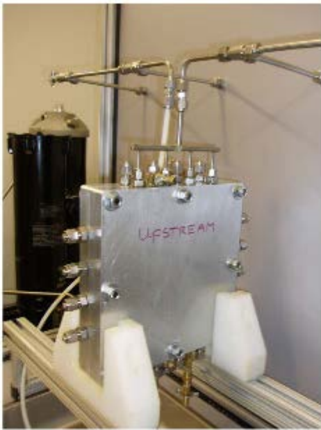
Fig. 1 Flatsheet media holder for fuel/water separation
